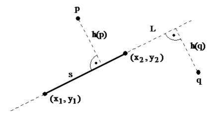
Exhibit 14.2: Segment s, its extended line L, and distance to points p, q as computed by function h.
