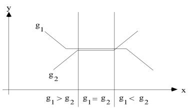
Exhibit 14.9: Desirable consistency condition for intersection of nearly parallel lines.
